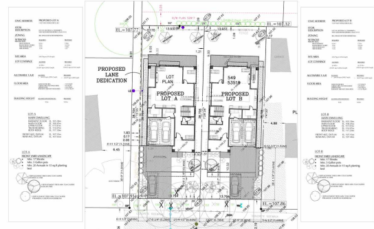
OVERALL SITE & LANDSCAPE PLAN 11607 88TH AVE DELTA B.C. 2 LOT SUBDIVISION SCALE: 1/8" = 1'-0" DATE: 05.10.2019 A-0
